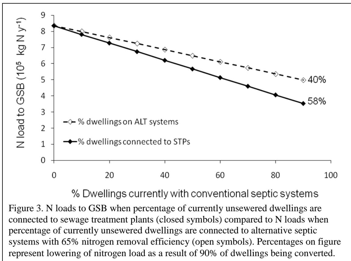
Not surprisingly, nitrogen loading was reduced more by sewerage than by use of alternative septic systems (Figure 3, Table 6). The maximum potential reduction in N load resulted from connecting dwellings to package sewage treatment plants. Wastewater was by far the largest contributor to total nitrogen load, and reductions in wastewater nitrogen had the largest effect on lowering total nitrogen load.
